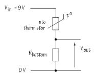
In this circuit when it is cold resistance of the thermistor is high.
